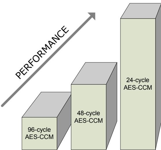
The smallest member of the family is the **"96-cycle" AES-CCM** core which takes a minimum 96-clock cycles to encrypt or decrypt each 16-byte data block using a 128-bit key.
