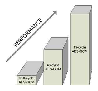
The smallest member of the family is the **"218-cycle" AES-GCM** core which takes a minimum 218 clock cycles to encrypt or decrypt each 16-byte data block using a 128-bit key.
